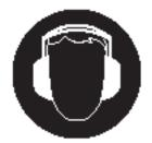
As the sound pressure level at the operator's ears exceeds 80 dB (A), ear protectors must be used when working with the machine to prevent hearing damage.
